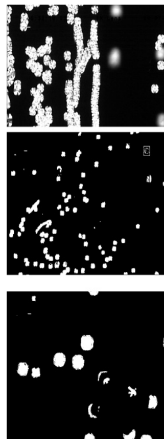
Figure 7. Morphological evidence of the decay in the number of nuclei on increasing the holding time after shear for unfractionated sample. The sample was sheared at 250 °C for 10 s at \dot{\gamma} = 30 \text{ s}^{-1} and held at this temperature for (a) t_R = 0 s, (b) t_R = 60 s, and (c) t_R = 180 s before isothermal crystallization at 180 °C.
